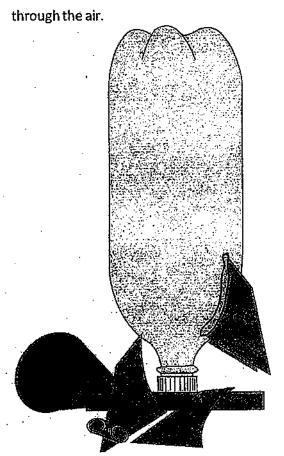
7. To create a nose cone you will need poster board or any other kind of strong material that you can roll into a cone that will fit over the bottom of the bottle. (Remember that the bottom of the bottle is now the top of the bottle when it is launched.) Once you roll your nose cone into shape, tape the edges so that it will stay together while it is flying. Now trim the bottom of the cone to fit the bottle and tape or glue the cone onto the bottle.
